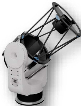
Figure 4. Model of the Planewave Instruments CDK700 telescope. Rotating tertiary mirror can direct the received light out along the elevation axis to the Nasmyth ports on either side of the telescope.
